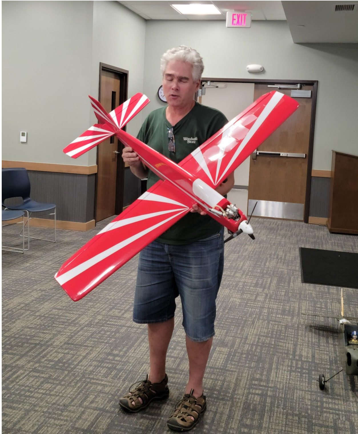
Matthew Mulbrook and his Hammer 25 with a Saito engine and a three-blade prop for ground clearance featured in Flying Models magazine.
