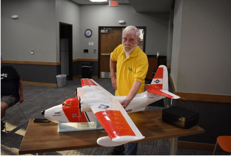
Gene Thorn brought in his “magnum opus.” This is the Grumman Albatross, which he has scratch built for both water and land use. He started it in September, 2022. He still has some trim work to do and to build the landing gear still. He said this is the hardest plane he has ever built due to complex curves and angles. It has a 72” wingspan runs on 2 850 Watt motors using 2 2200mAh 3 cell batteries.
