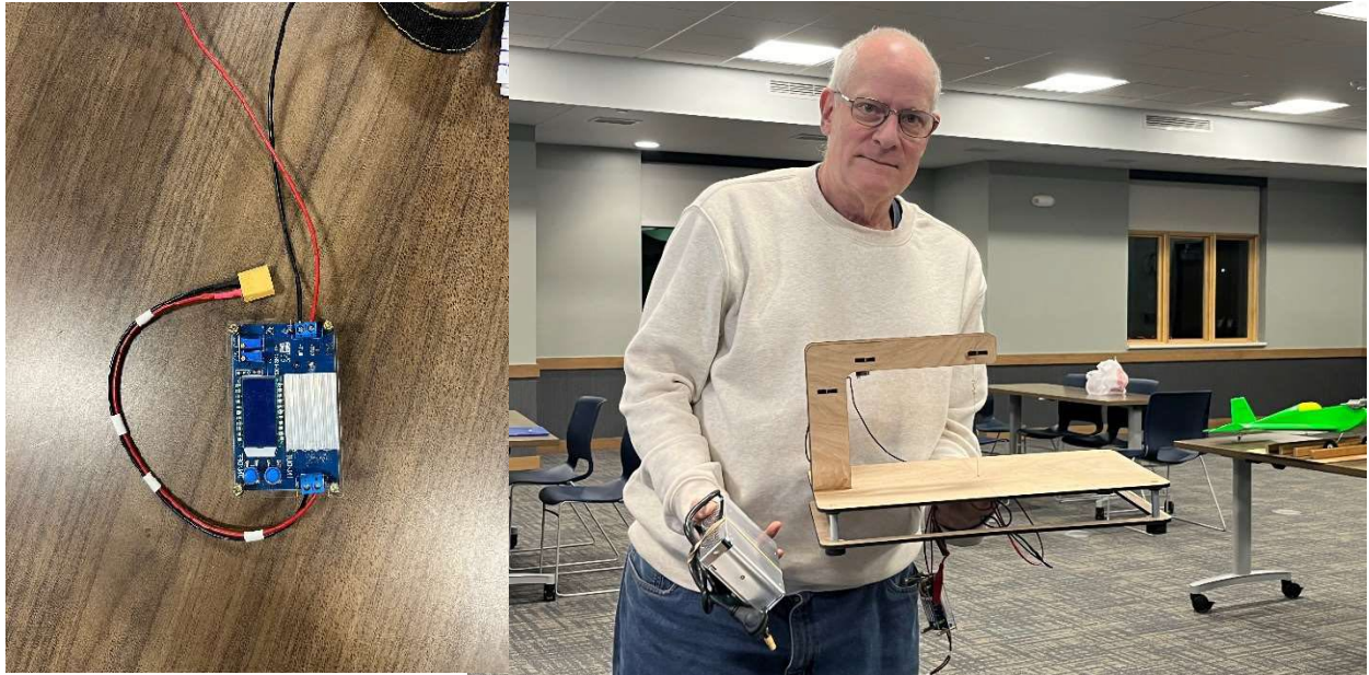
Figure 3-Don Rosendale brought in a homemade foam hot wire cutter. He used feathercut wire. He purchased a power supply on Amazon that can control voltage and current.
