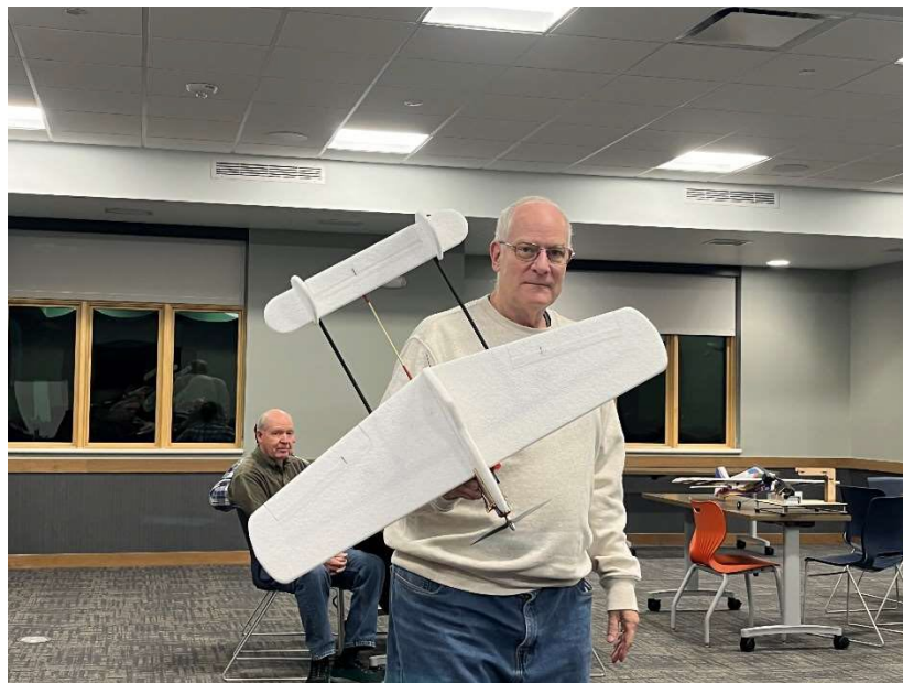
Figure 2-Don Rosendale showed a plane called the Funder and Lightning. It is being built as a club project with the Quiet Flyers. The plans are available on RC Groups. He is using a 2213 KV motor with a 1300 mAh battery and a 40 Amp speed controller.
