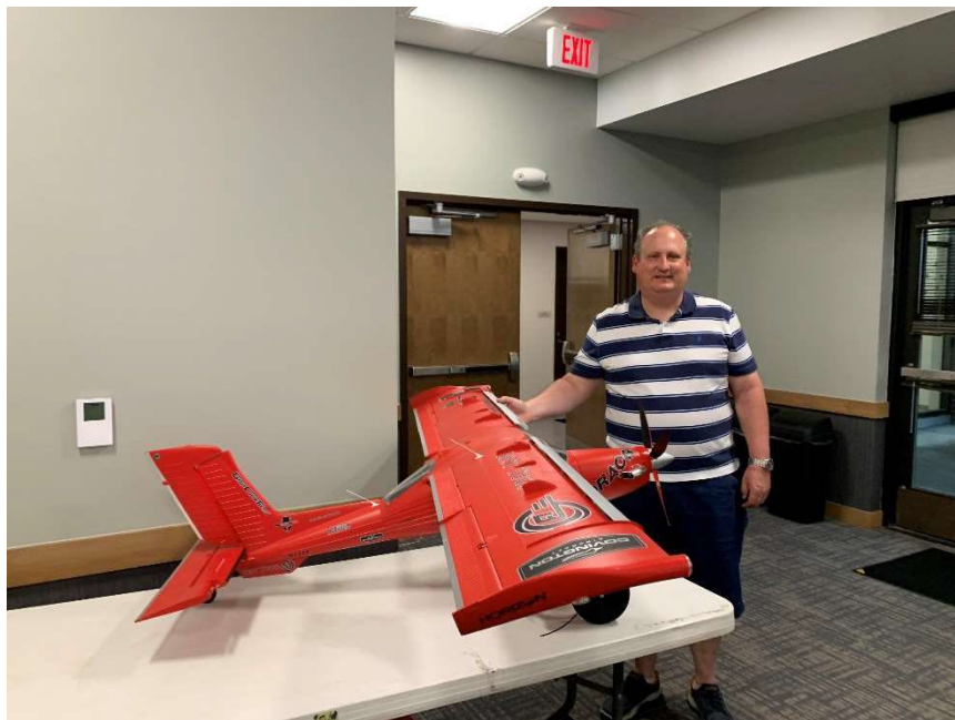
Figure 1-Jim Doty brought in his recently completed Horizon Hobby BNF Draco. It comes with LED lighting and a brushless motor. It runs on 6S 5000 mAh battery pack.
