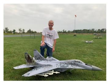
Gary Owen brought his new jet to show. It is a Freewing MiG-29 with twin 80 mm EDFs. It has been highly modified from the stock ARF as it has dual axis thrust vectoring, thrust reversers and LED afterburners. It runs on dual 6S LiPo batteries and it is equipped with GPS telemetry. The jet is controlled by a Graupner radio using 16 channels.
