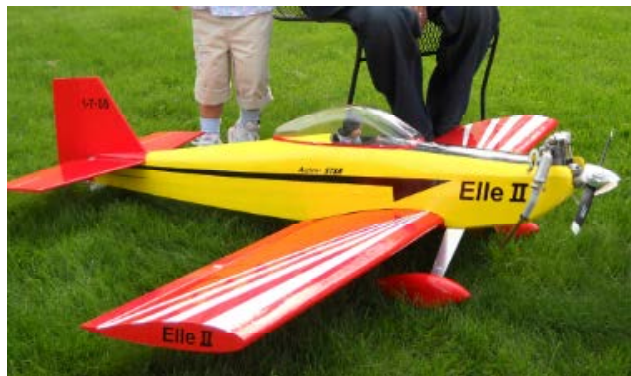
SIG Astro-Hog - "Elle II" Length: 52.5 in., Wingspan: 60 in. Engine: Glow Saito 100 4-stroke
