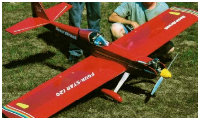
SIG Four-Star 120 - "Donnybrook" Length: 63 in., Wingspan: 74.5 in. Engine: Glow O.S. 120 with Pump 4-stroke
