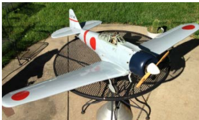
Top-Flite "Hollywood Zero" Length: 50 in., Wingspan: 72 in. Engine: Glow Super Tigre 90 2-stroke
