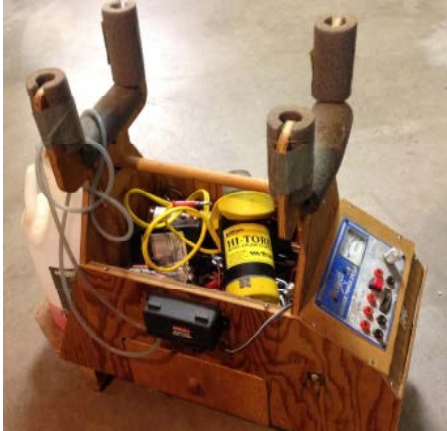
Field Box Includes: Starter, Fuel Pump, Small Tools, Etc.
