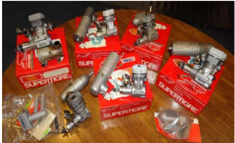
Back Row left-right: STG61ABC w/ in cowl muffler, STG40 Ring w/ muffler, STGS45 ABC w/ muffler and extension, STG90 Ring w/ muffler
