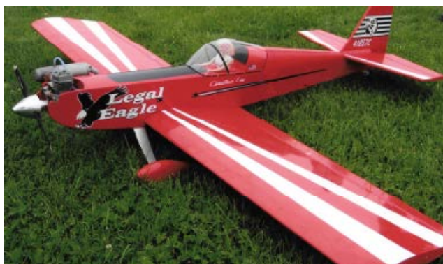
SIG Four-Star 60 - "Legal Eagle" Length: 55 in., Wingspan: 71 in. Engine: Glow Super Tigre 75 2-stroke
