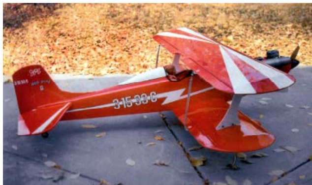
SIG Hog Bipe - Length: 48 in., Wingspan: 54 in. Engine: Glow Super Tigre 61 2-stroke
