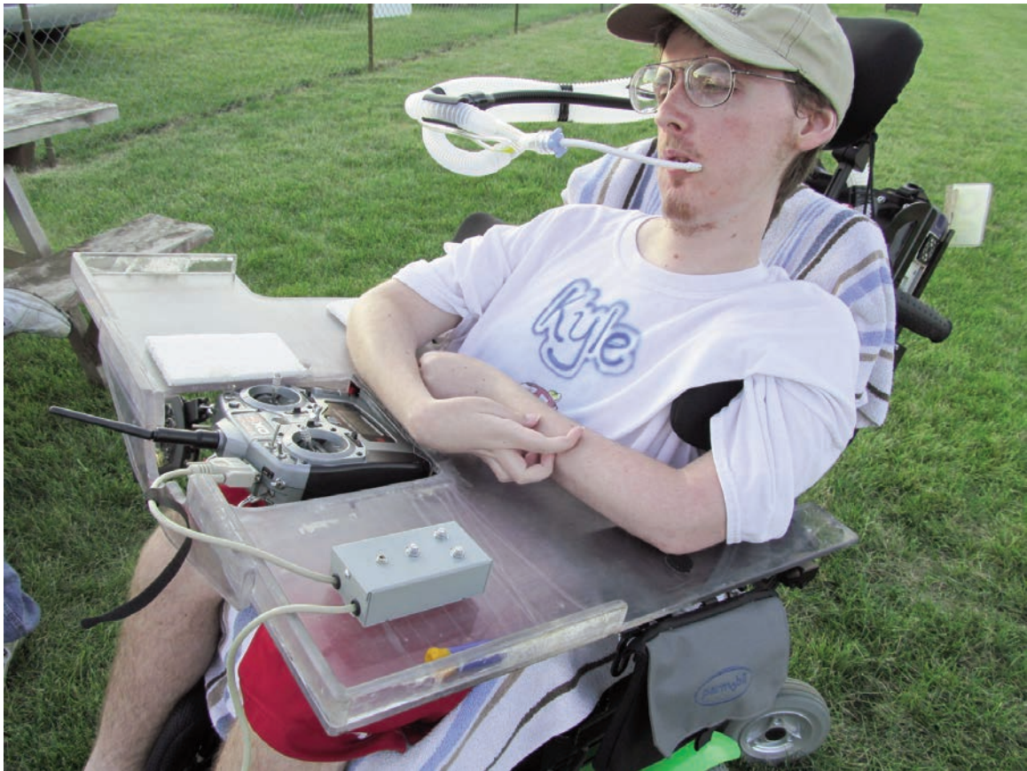
Kyle Smart's "toe control" for rudder operation, designed and built by Kyle's dad, Joel and Rich Dean
